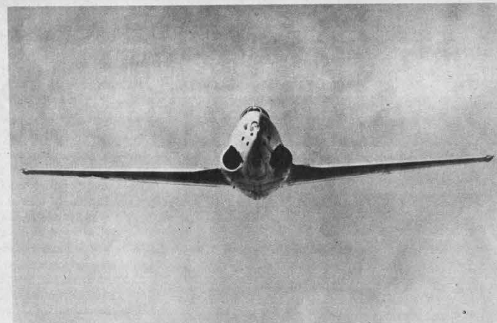
Seen head-on, P-80's nose looks like bleached skull of a horned animal. Openings between air intakes are for a landing light and six .50-caliber MG's. Slight wing dihedral stems from roots.
